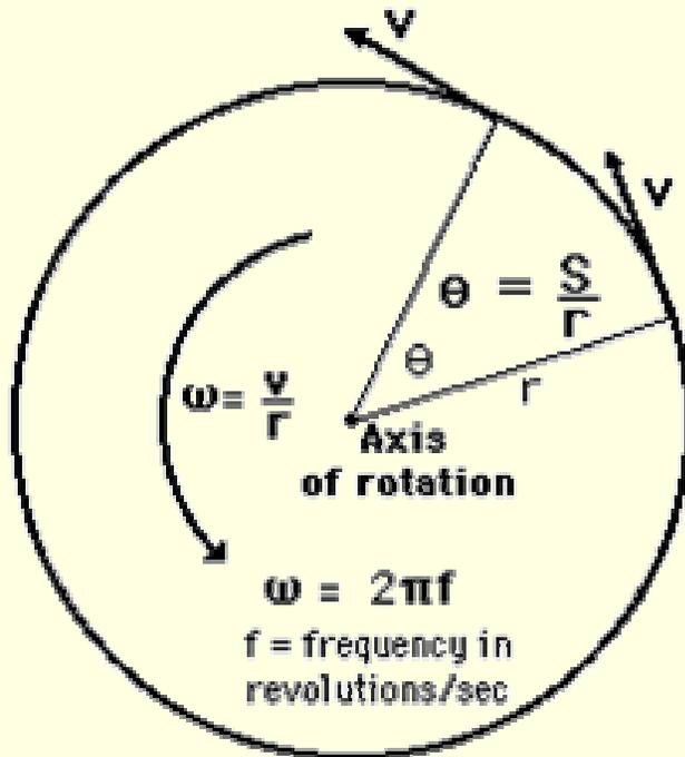
Angular velocity can be considered to be a vector quantity, with direction along the axis of rotation in the **right hand rule** direction.
