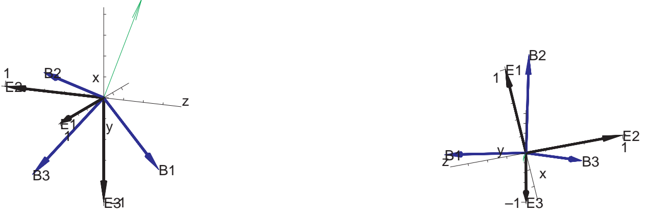
Figure 4.1. Rotation interpreted in (\mathbf{v}, \Phi) context for (\phi, \theta, \psi) = (\pi/6, \pi/6, \pi/3) . Left view: \mathbf{v} (regular arrow) overlaid on Figure 2.1. Right view: Looking down \mathbf{v} .
