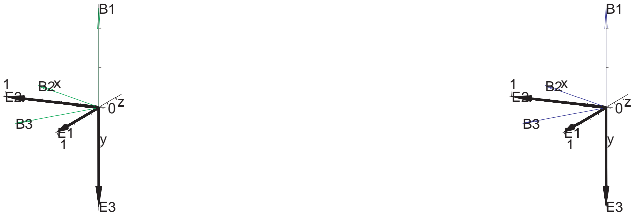
Figure 2.4. Degeneracy of Euler-angle decomposition for \theta = \pi/2 . At left: (\phi, \psi) = (2\pi/3, \pi/2) . At right: (\phi, \psi) = (\pi/3, \pi/6) .
